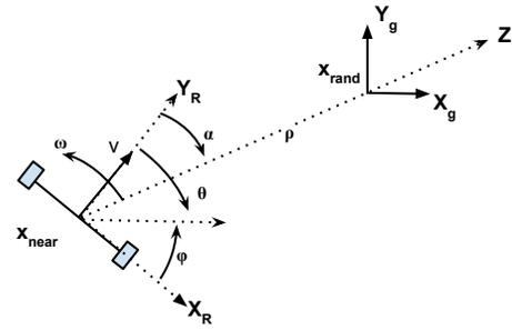
Fig. 2. Robot and goal pose relations and notation
