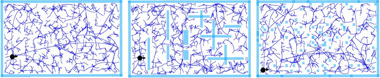
Fig. 6. Example trees obtained using the Euclidean distance in the three scenarios. The initial pose of the robot is shown by a black dot. Although state space coverage is good, the planner generates trees that lead to poor solutions in terms of path length and quality.
