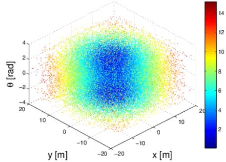
Fig. 4. The cost-to-go function  $C(\mathbf{0}, \mathbf{x})$  for paths generated by the POSQ controller.
