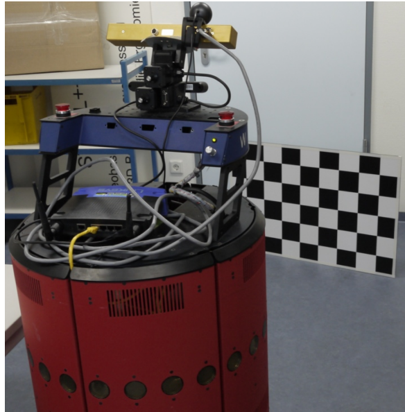
Figure 3: The Robot collects data using the stereo camera and the laser range finder. The calibration pattern is visible from both sensor modalities.
