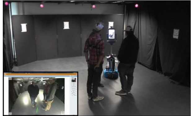
Fig. 1. Example of the interactions described in the paper. A group of four participants discuss a murder mystery. One of them is remotely present through a robot, and has to go through several approach/converse/retreat cycles. The inset shows the interface as seen by this participant.
